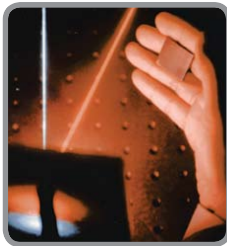
■ The coating technique will use three laser systems: a resonance absorption laser, a UV laser and a controlled plasma cooling and coating formation laser.
