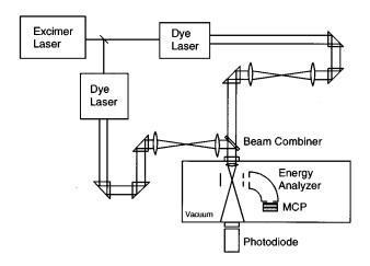
FIG. 2. Schematic diagram of the experimental layout.
