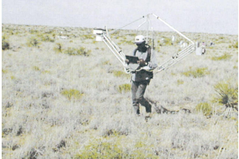
Figure 7. A researcher from the University of Arizona collects multispectral radiometer data over a field transect.
