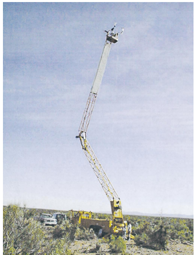
Figure 3. The 30-m boom extended from the truck at the transitional land-cover area. At the top of the boom are two instruments for measuring sky and surface radiance, a modified Cimel sunphotometer (NASA GSFC), and PARABOLA III (JPL).
