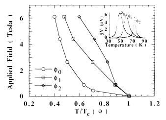
FIG. 4. Irreversibility line before  $(\phi_0)$  and after irradiation at  $\phi_1 = 1 \times 10^{11}$  and  $\phi_2 = 3 \times 10^{11}$  ions/cm<sup>2</sup>. Inset: The quadrature  $(\chi^{\parallel})$  component of the pickup voltage at 4.4 T before and after irradiation.
