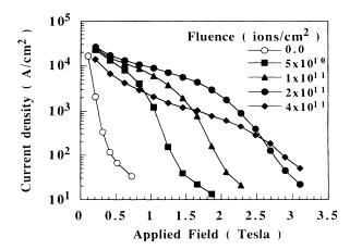
FIG. 3. Critical current density plotted as a function of applied field (H||c). The data were taken at 77 K.
