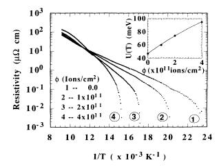
FIG. 2. The resistivity data at 5 T (H||c) before and after irradiation. Inset: A plot of the activation energy at 77 K vs  $\phi$ .
