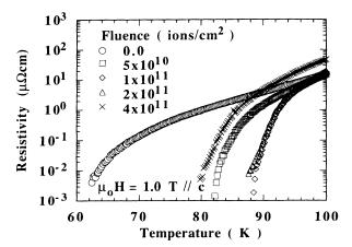
FIG. 1. Electrical resistivity of a TI-2:2:2:3 film before and after irradiation with the Ag ions. The data were taken at 1 T (H||c).
