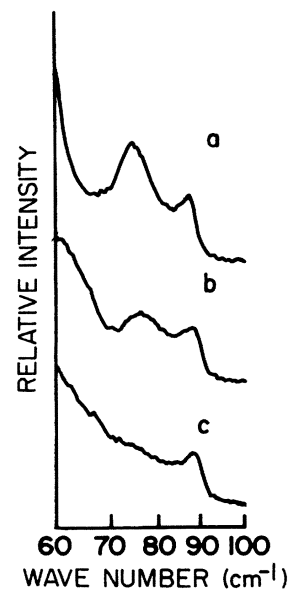
FIG. 7. Behavior of 83\text{-cm}^{-1} line ( 75\text{ cm}^{-1} at 300\text{ K} ) on heating through T_c : (a) 300\text{ K} , (b) 373\text{ K} < T < 432\text{ K} = T_c , (c) T > 432\text{ K} .
