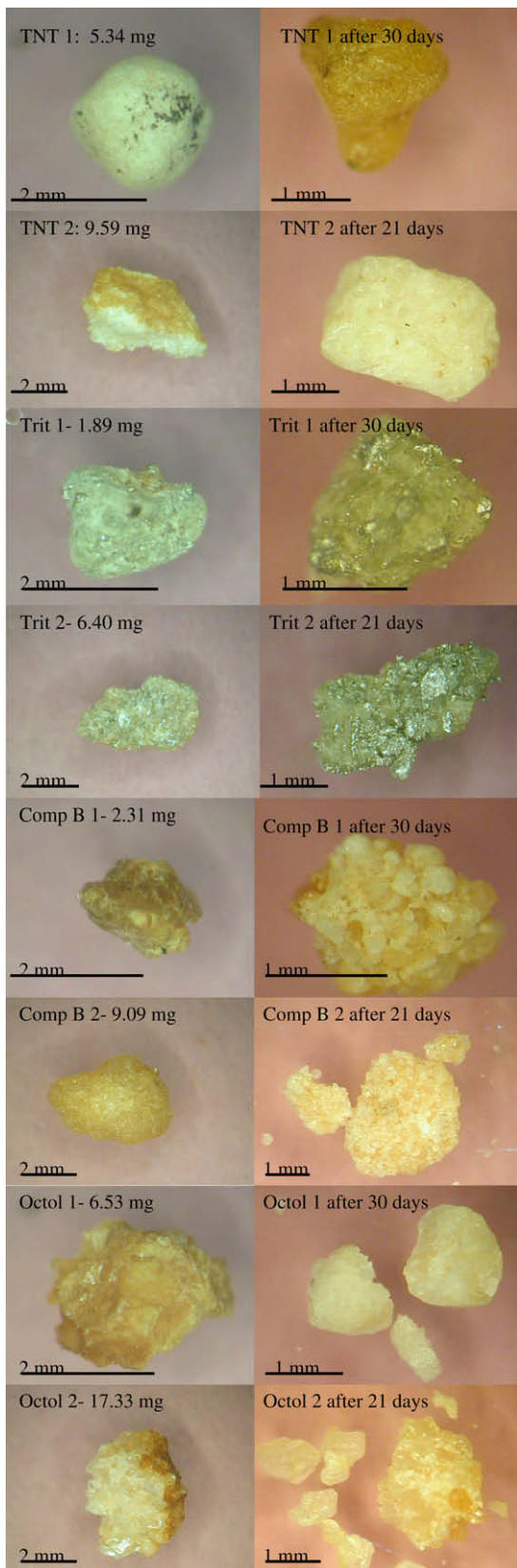
Fig. 1. Photos and initial masses of mm-sized particles used in the laboratory tests paired with photos of the same particle taken partway through the tests.
