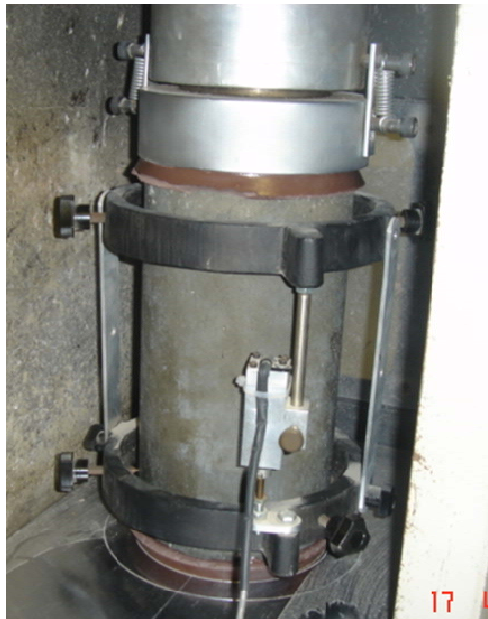
Figure 4.13: Capped 6x12 in. cylinder fitted with electronic combined compressometer and extensometer
