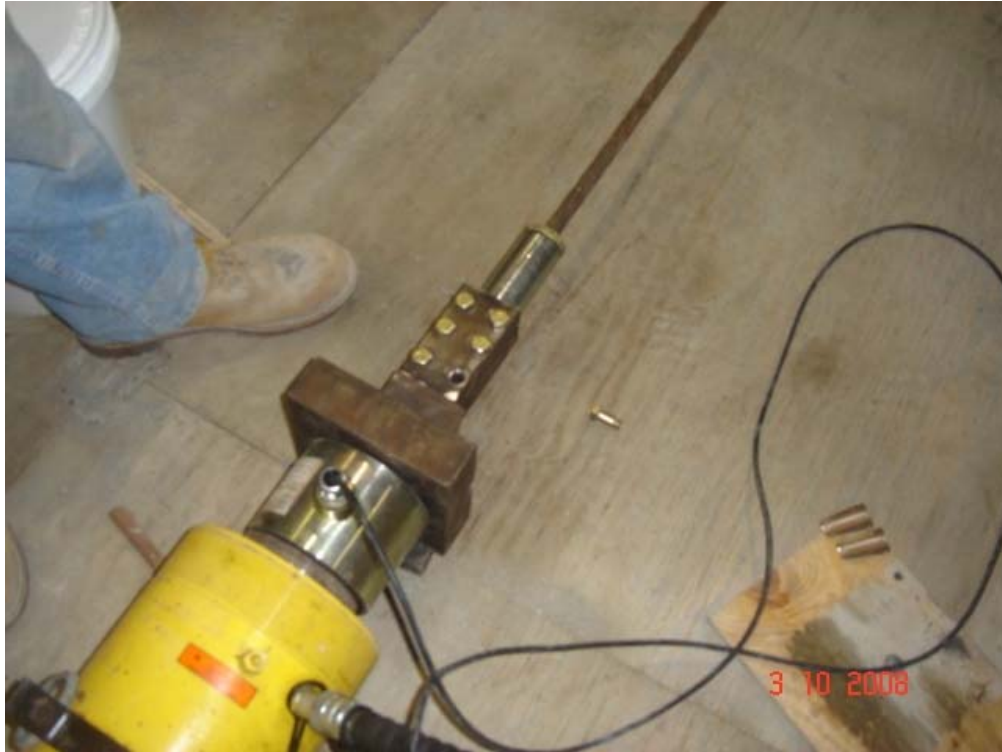
Figure 3.13: Pullout test setup (gripping technique #2)
