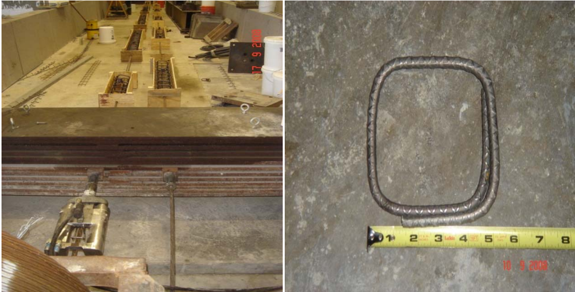
Figure 3.7: Pretension specimen rows (form work and confining)
