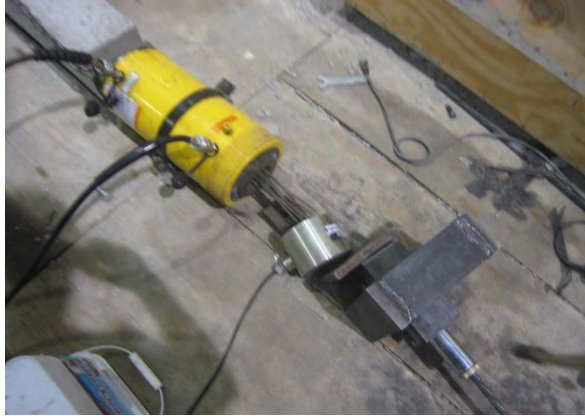
Figure 3.19: Strand rupture @ stress \geq 270 ksi
