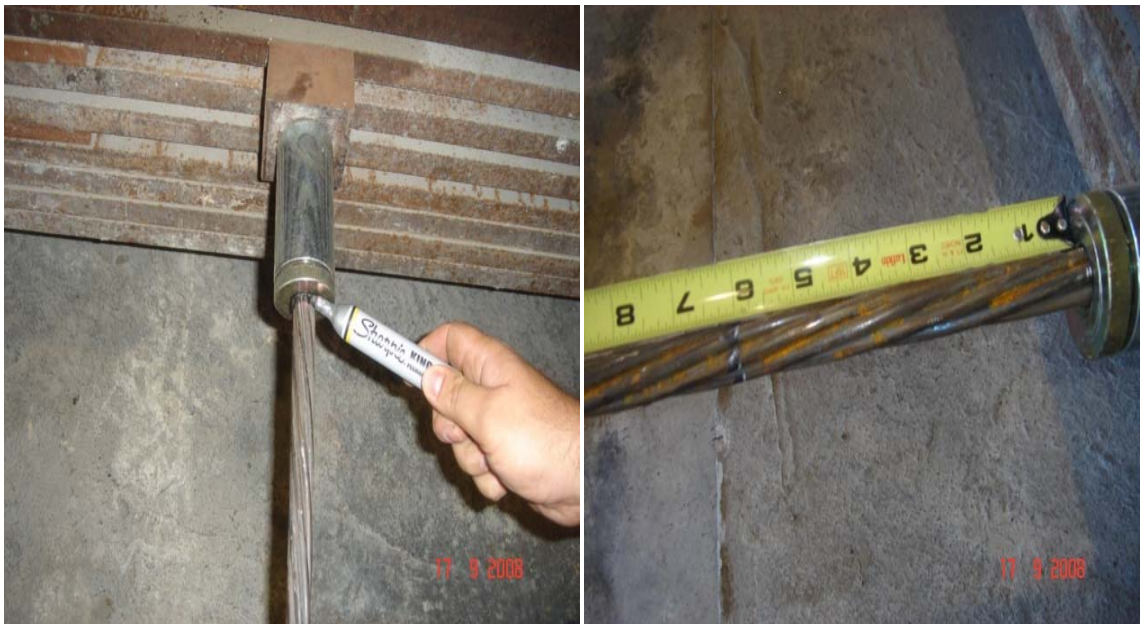
Figure 3.8: Marking and measuring the strand elongation
