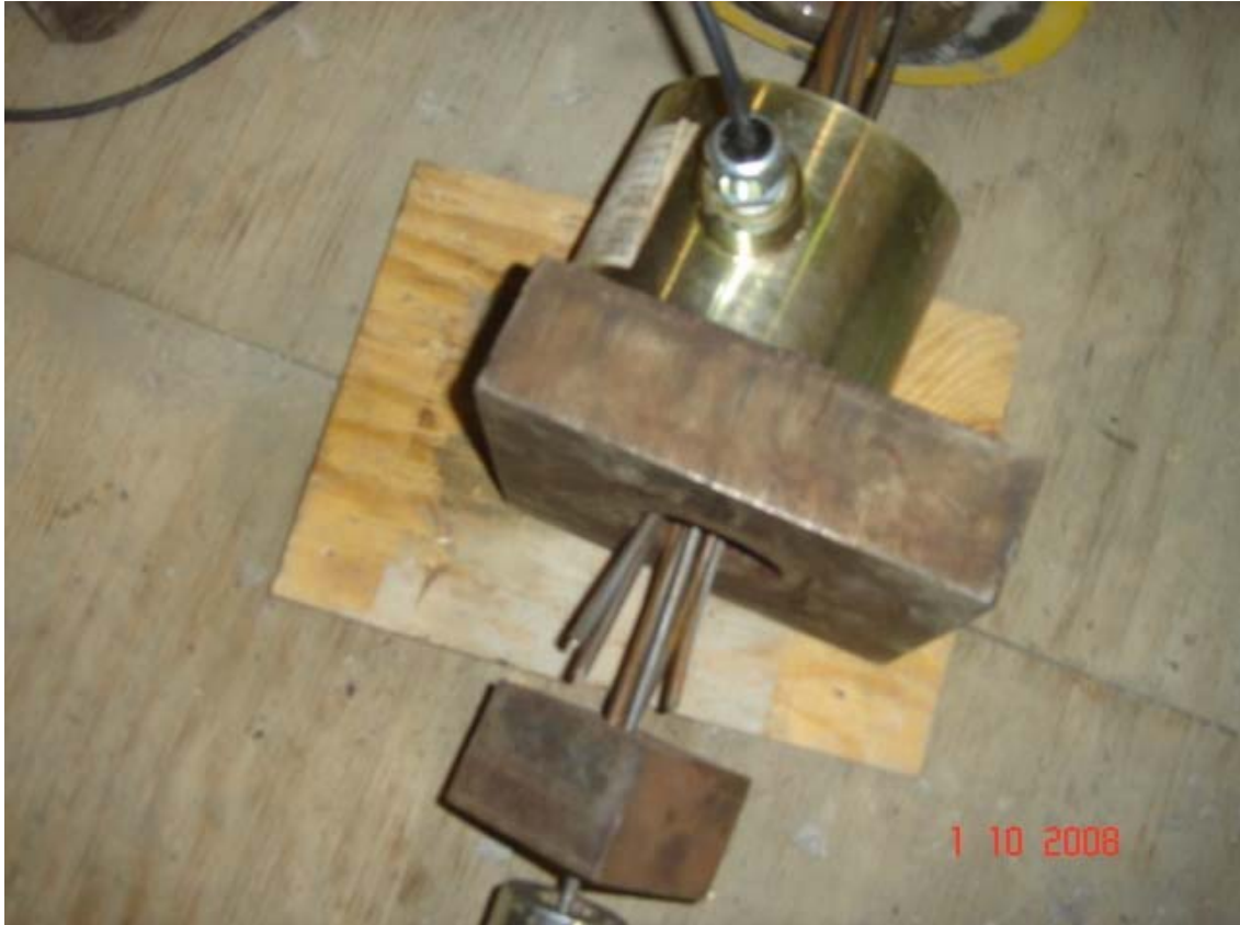
Figure 3.12: Strand failure at the chuck location
