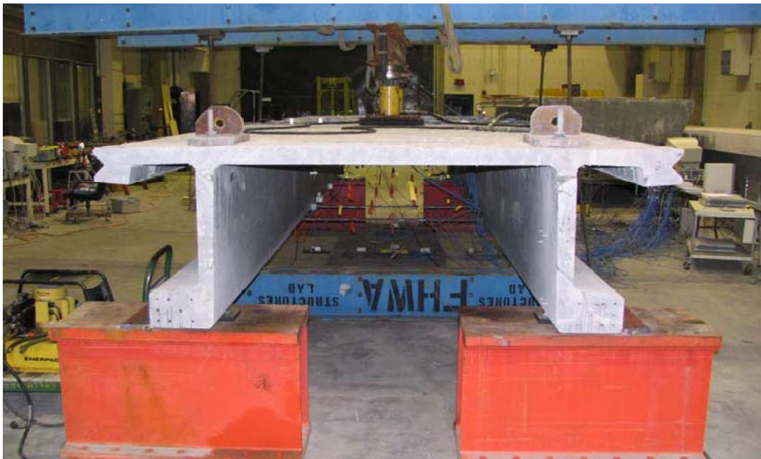
Figure 4.4: Pi-girder testing at TFHRC (Keierleber et al.)
