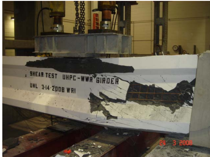
Figure 5.11: Shear cracks at failure of AASHTO Type II girders
