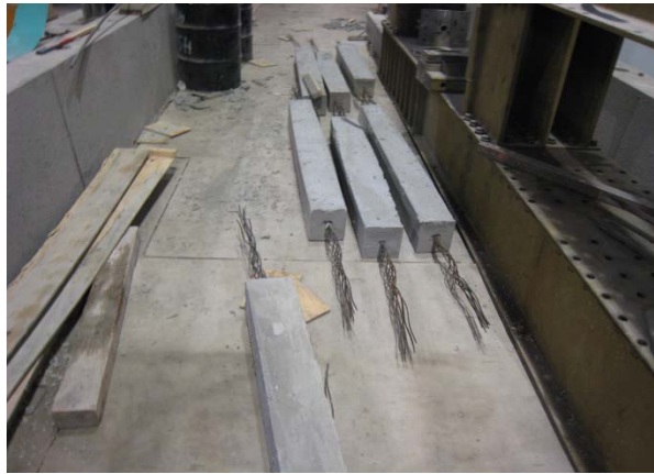
Figure 3.20: Specimens set#1 strand rupture
