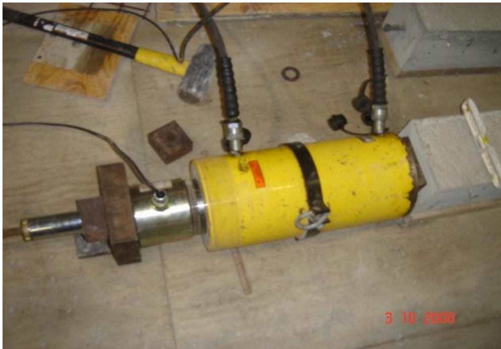
Figure 3.11: Pullout test setup (gripping technique #1)
