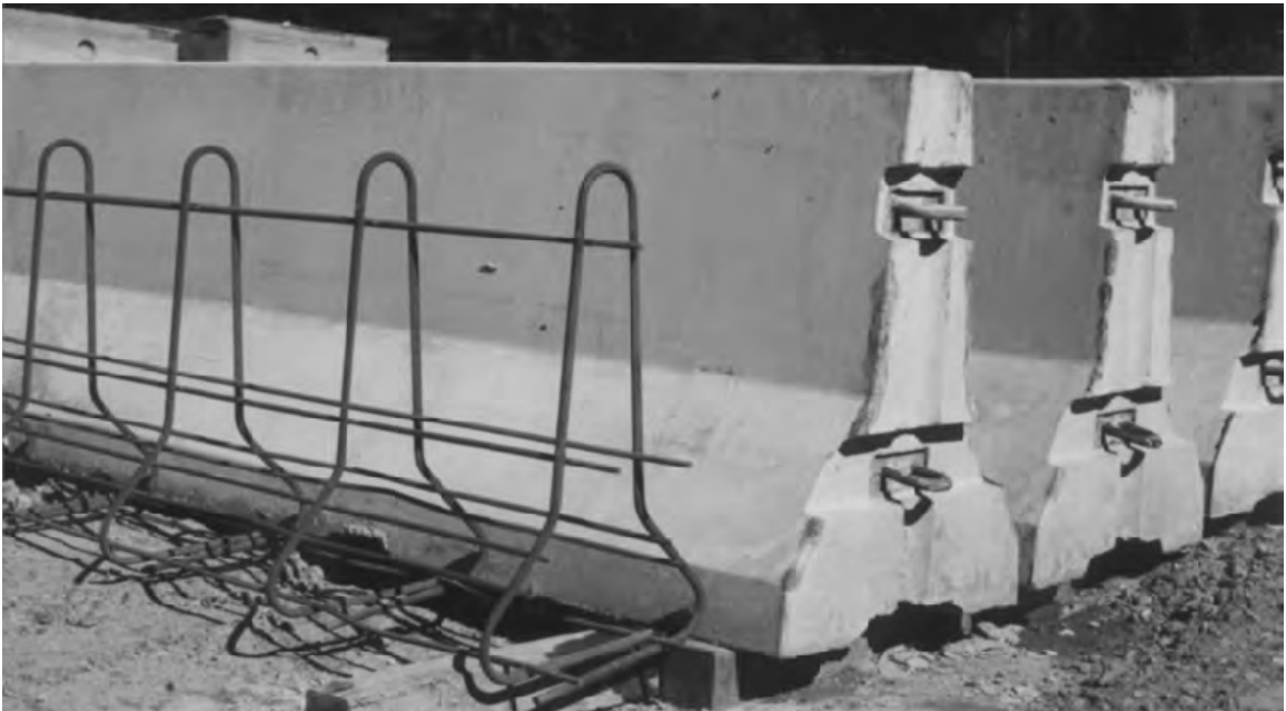
Figure 5.2: WWR used in fabricating highway median barriers (WRI Manual of Standard Practice, 2006)
