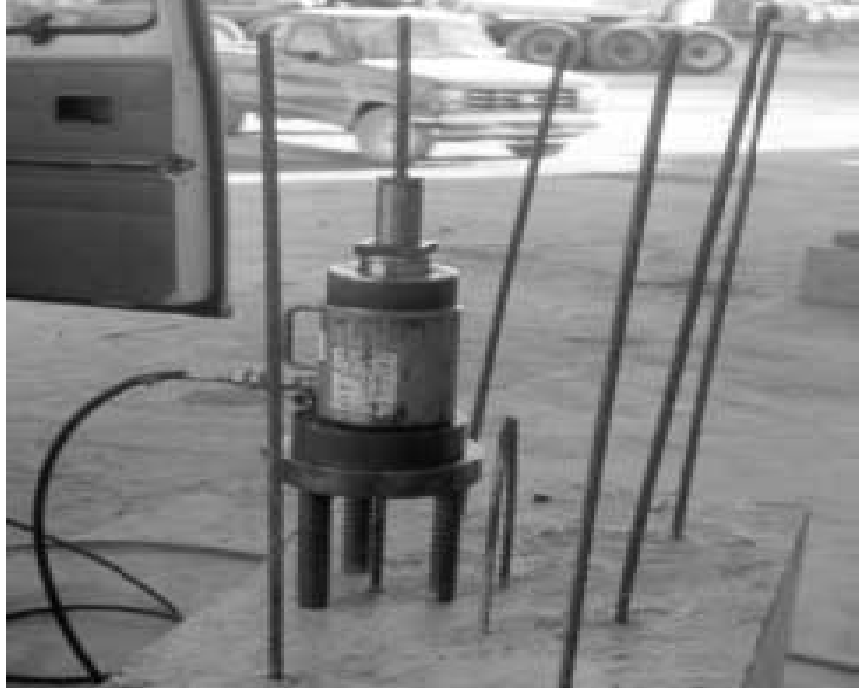
Figure 2.12: Pullout test setup (Barnes et al. 1999)
