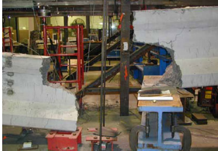
Figure 4.2: Girder failure (Publication No. FHWA-HRT-06-115)
