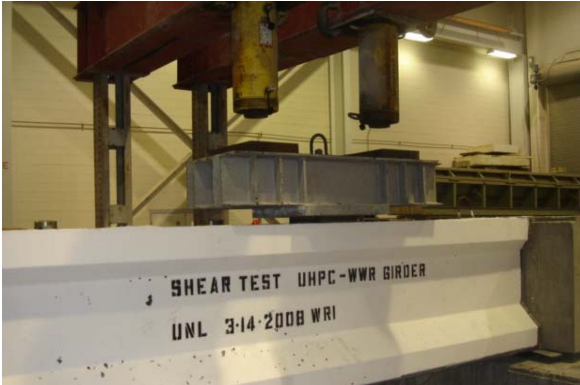
Figure 5.8: Shear test setup – girder A
