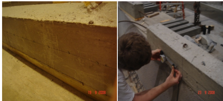
Figure 3.26: Performing a measurement using a DEMEC gauge
