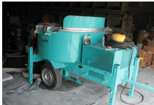
Figure 4.7: High energy paddle mixer – University of Nebraska Lab
