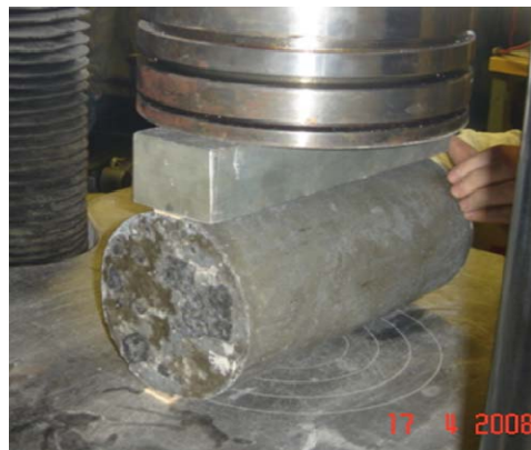
Figure 4.15: Split cylinder cracking strength test set-up
