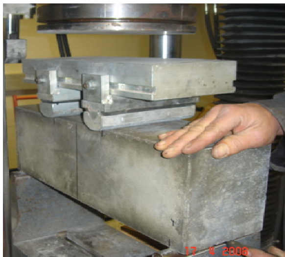
Figure 4.17: Modulus of rupture test setup
