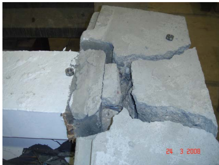
Figure 5.12: Diaphragm failure at ultimate capacity
