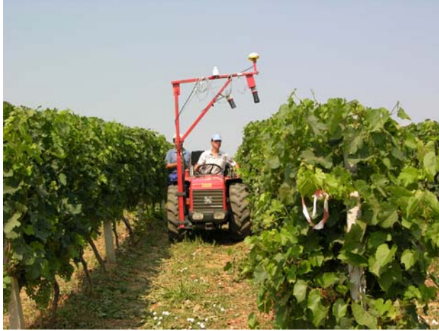
Fig. 2 Configuration of the mobile system with two down-facing passive sensors (near-vertical and oblique viewing angles) coupled with an up-facing sensor and a differential GPS
