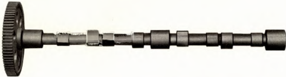
Cam shaft showing driving gear attached. There are three bearings having a total length of 7\frac{1}{2} in. Diameter of shaft 2\frac{2}{5} in.
