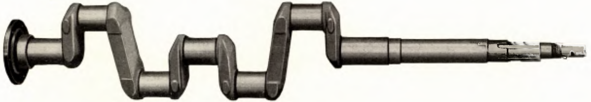
Extra large crank shaft, 2\frac{3}{4} in. diameter, turned and ground. It has three bronze-back babbitt lined bearings. Total length of bearings 12 in.
