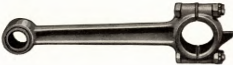
The connecting rod is 14 in. long, drop forged and heat treated. The cap on crank end of rod is held in place by four heavy steel bolts, insuring safety and more permanent adjustment.
