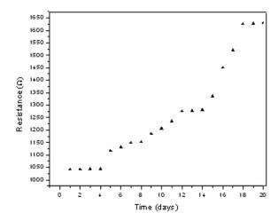
**Figure 4.** The resistance of semiconducting boron carbide with time, at room temperature under exposure to a mercury vapor.
