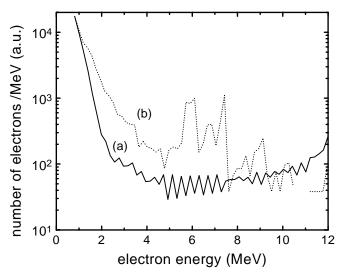
**FIGURE 7.** Simulational result of electron energy spectrum for different channel radii at  $\epsilon = 0.15$ ,  $r_0 = 5 \ \mu\text{m}$ ,  $\omega_p = 3.4 \times 10^{14} \ \text{rad/s}$ ,  $T_{ez} = 200 \ \text{keV}$ , and  $L = 400 \ \mu\text{m}$ : (a)  $r_0 = 500 \ \mu\text{m}$ , and (b)  $r_0 = 5 \ \mu\text{m}$ .
