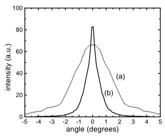
**FIGURE 6.** Simulational result of angular profile of the electron beam for different field amplitudes at  $r_0 = 5 \ \mu\text{m}$ ,  $\omega_p = 3.4 \times 10^{14} \ \text{rad/s}$ ,  $T_{ez} = 200 \ \text{keV}$ , and  $L = 400 \ \mu\text{m}$ : (a)  $\epsilon = 0.3$ , and (b)  $\epsilon = 0.15$ .
