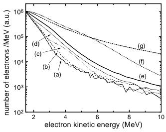
**FIGURE 2.** Electron energy spectra for different peak laser powers and plasma densities: (a) 2.6 TW,  $3.4 \times 10^{19}$  cm<sup>-3</sup>, (b) 2.9 TW,  $3.5 \times 10^{19}$  cm<sup>-3</sup>, (c) 3.3 TW,  $4.8 \times 10^{19}$  cm<sup>-3</sup>, (d) 3.9 TW,  $4.8 \times 10^{19}$  cm<sup>-3</sup>, (e) 1.7 TW,  $6.2 \times 10^{19}$  cm<sup>-3</sup>, (f) 2.7 TW,  $6.2 \times 10^{19}$  cm<sup>-3</sup>, , and (g) 3.5 TW,  $6.2 \times 10^{19}$  cm<sup>-3</sup>.
