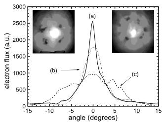
**FIGURE 1.** Lineouts of the electron beam profiles for different peak laser powers and plasma densities: (a) 2.9 TW,  $3.4 \times 10^{19} \text{ cm}^{-3}$ , (b) 3.5 TW,  $6.2 \times 10^{19} \text{ cm}^{-3}$ , and (c) 0.6 TW,  $2.3 \times 10^{19} \text{ cm}^{-3}$ . Inset on the left side shows the electron beam profile at 3.5 TW and  $6.2 \times 10^{19} \text{ cm}^{-3}$ . Inset on the right side shows the electron beam profile at 2.0 TW and  $2.3 \times 10^{19} \text{ cm}^{-3}$ .
