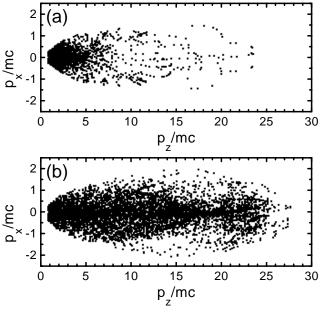
**FIGURE 5.** Simulational result of momentum distribution of electrons injected over the entire 400- $\mu$ m-long channel for different field amplitudes at  $r_0 = 5 \ \mu$ m,  $\omega_p = 3.4 \times 10^{14} \ \mathrm{rad/s}$ , and  $T_{ez} = 200 \ \mathrm{keV}$ : (a)  $\epsilon = 0.15$ , and (b)  $\epsilon = 0.3$ .
