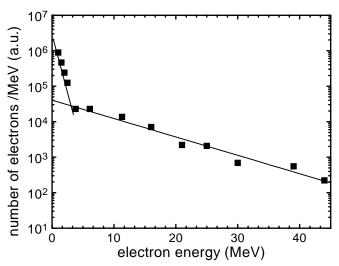
**FIGURE 3.** Electron energy spectrum for 3-TW peak laser power and  $3 \times 10^{19}$ -cm<sup>-3</sup> plasma density.
