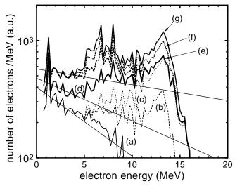
**FIGURE 8.** Simulational result of electron energy spectrum for different channel lengths at  $\epsilon = 0.3$ ,  $r_0 = 5 \mu \text{m}$ ,  $\omega_p = 3.4 \times 10^{14} \text{ rad/s}$ , and  $T_{ez} = 200 \text{ keV}$ : (a) 54, (b) 109, (c) 163, (d) 218, (e) 272, (f) 327, and (g) 381 $\mu \text{m}$ .
