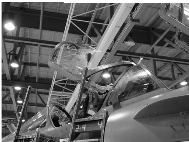
Figure 2: Two examples of canopy damage to military aircraft caused by Osprey .
