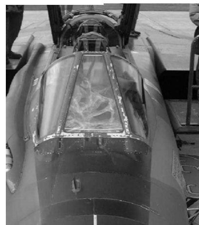
Figure 2: Two examples of canopy damage to military aircraft caused by Osprey .
