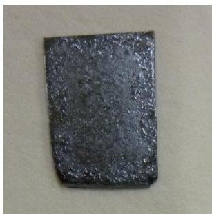
Figure 6. Picture of a fresh film composed of HDTMS and TMOS dropcasted onto a silicon wafer, tg = 30minutes
