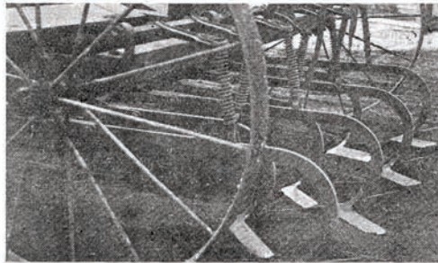
FIG. 2.—View of the duck-foot or sweep cultivator used in the Experiment Station tests, showing the overlapping arrangement of the shovels.
