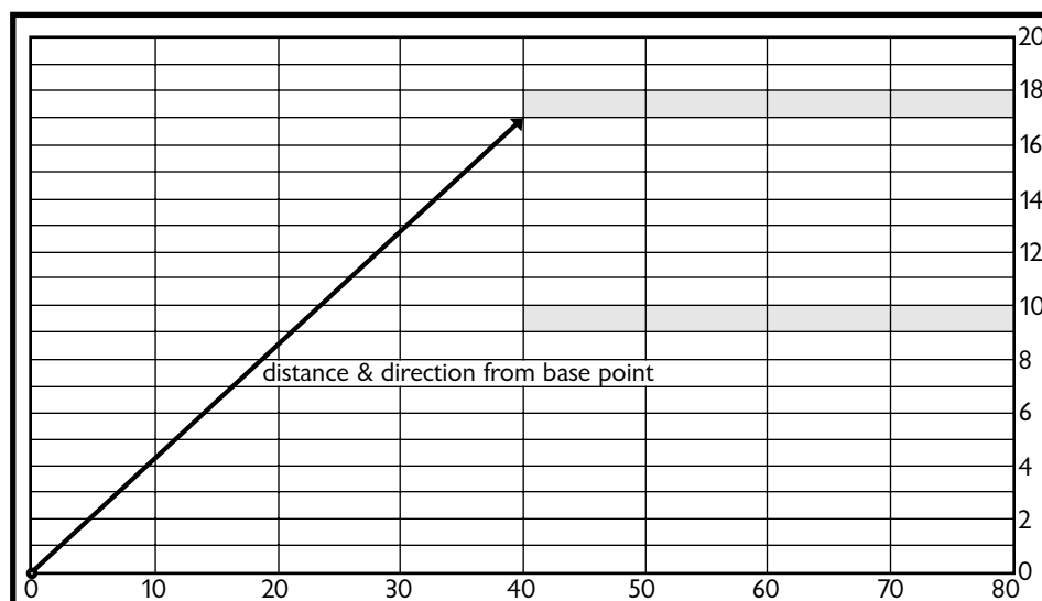
FIGURE 8.11. Sampled area gridded into sampling unit locations (potential plot placements). Plots can be located by pacing or measuring from base lines at the edges of the area to be sampled or by converting x-y coordinates into distance and azimuth from a single base point.
