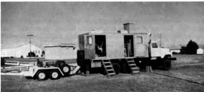
Fig. 1. Photo of penetrometer truck and developed for investigation of hazardous waste sites.
