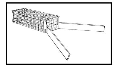
Figure 1. Diagram of the unbaited trap with wings used to capture nine-banded armadillos in South Georgia, summer 2004. Wings were constructed of pressure-treated lumber (2" x 6" x 6").
