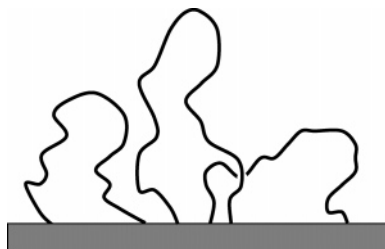
Figure 7. Schematic representation illustrating how variations in distances between tethering points and chain crossover affect the ability of the tethered loops to extend normal to the surface. The net result is that the layer appears to be comprised of loops of different sizes; this effect is referred to as an “anchor-induced” polydispersity.
