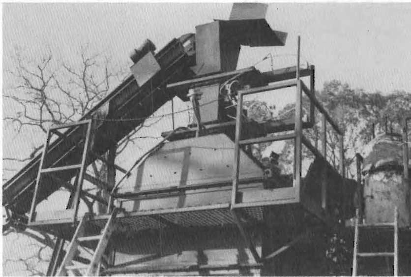
Figure 4. Close-up view of conveyer and input system--EES pyrolysis pilot plant.
