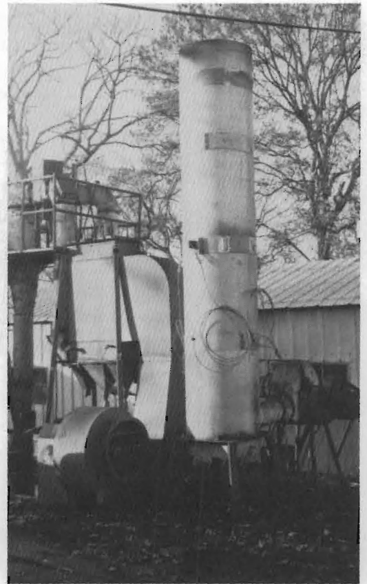
Figure 6. Close-up view of off-gas burner--EES pyrolysis pilot plant.
