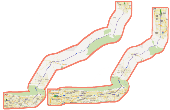
Figure 11. Compressing the highway between Las Vegas and Los Angeles. Left: original route cut from surroundings. Right: route transmogrified to show more details around cities and less across the desert.
