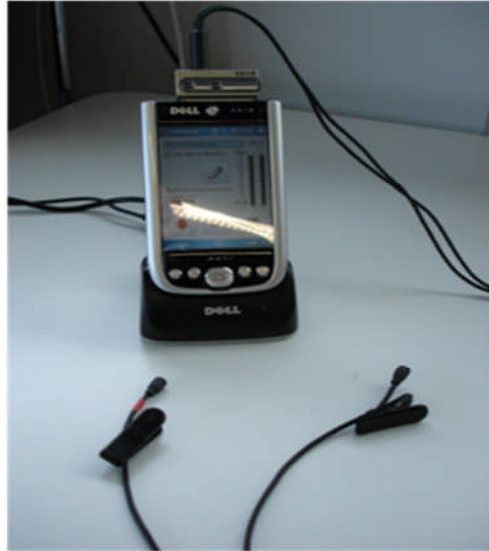
Figure 5. Binaural recording device used to record and analyse the CT ward soundscape.
