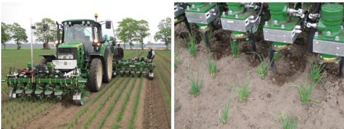
Figure 7: Robocrop used in field on planted seedling of onion in small groups.
