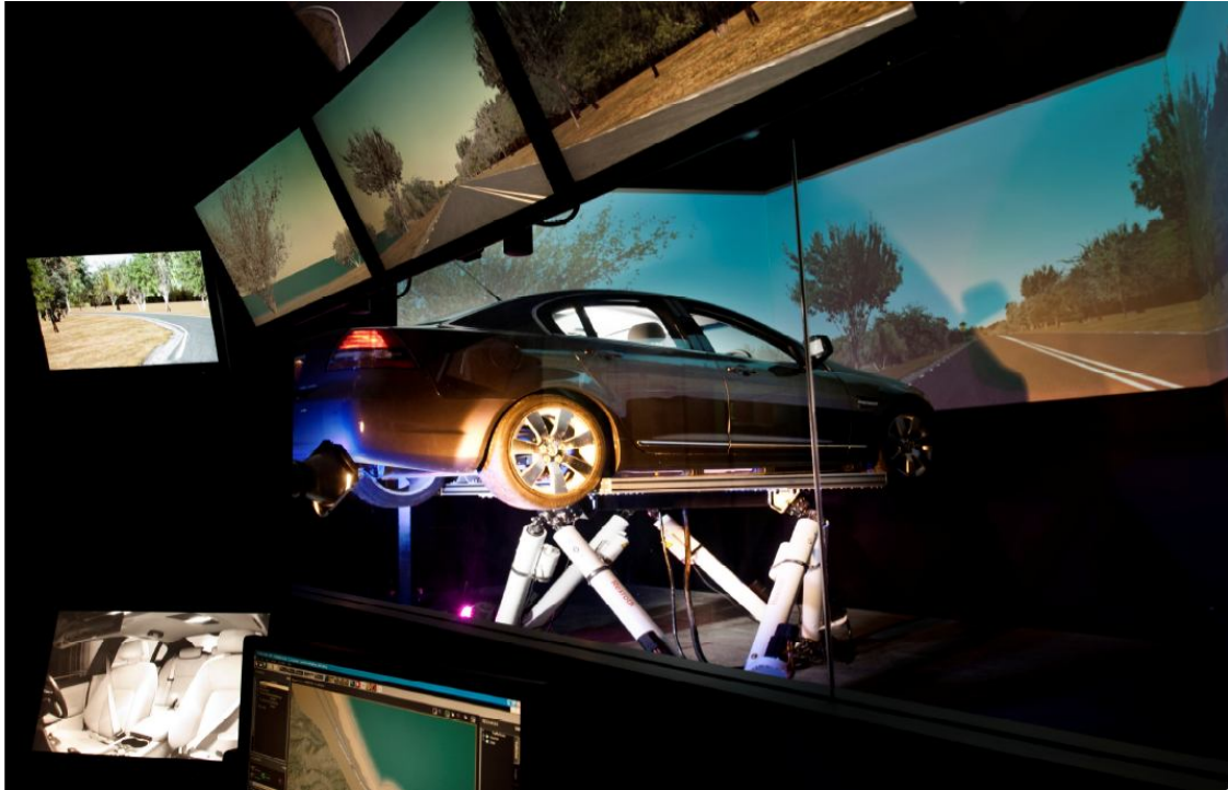
Figure 1 Driving simulator at Carrs-Q
