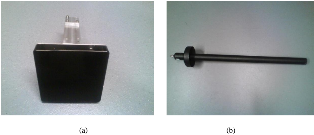
Figure 2.6: (a) HC low-gain antenna, (b) RC helical antenna
