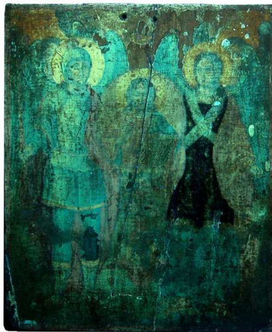
Figure 4. UV fluorescent image of the coated surface showed a green-yellow emission that indicated the presence of an aged natural resin varnish. The non-fluorescent dark areas and back spots indicated the presence of soiling depositions.
