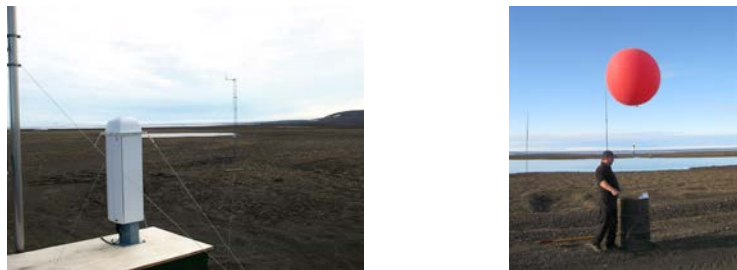
Figure 2. Ceilometer and the 10 m mast for flux and air quality measurements in the left panel. Releasing radio sonde, right panel.
