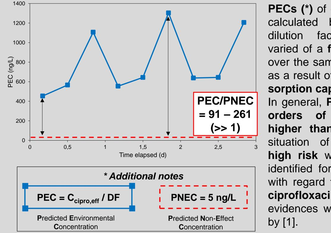
**PECs (\*)** of ciprofloxacin, calculated by using a dilution factor **DF=10**, varied of a factor of ~ 3 over the sampling period, as a result of changes in sorption capacity. In general, PECs were 2 orders of magnitude higher than PNECs. A situation of **potentially** high risk was therefore identified for Bekkelaget, with regard to release of ciprofloxacin. Similar evidences were obtained
