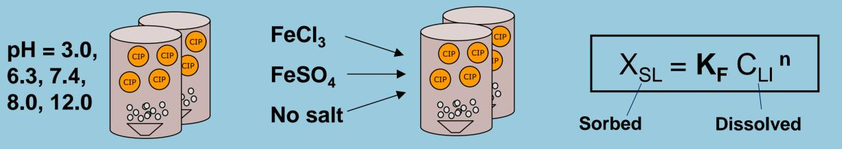
2) The Activated Sludge Model for Xenobiotics – ASM-X ([7]) was used to predict measured ciprofloxacin's concentrations at Bekkelaget WWTP (Oslo). Freundlich parameters estimated in batch were used for ASM-X calibration. Effluent concentrations of ciprofloxacin (C<sub>cipro,eff</sub>) could also be estimated.
