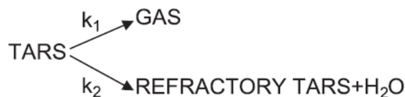
Figure 2.14: A global mechanism for the secondary reactions of vapor-phase tarry species 4
