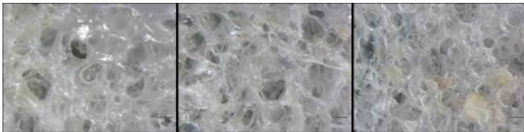
Fig.7 Optical micrographs of the PIM sample core (from left to right) M04, M15, and M13, with 5, 10 and 15 wt % sand showing its effect on pore sizes.
