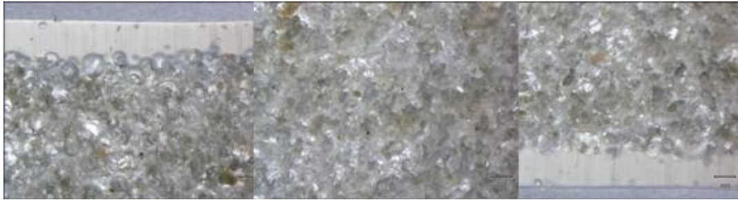
Figure 6: Optical micrographs of cross section of the PIM samples M16 with 80 wt% PE (LDPE/HDPE=90/10) and 10 wt% sand and 10 wt% rPET (from left to right: the top skin, the core, and the bottom skin).
