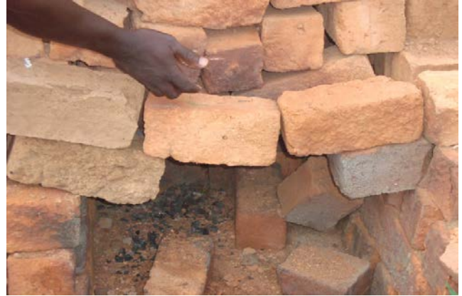
Plate 8: Stacked burnt bricks around firing channel
