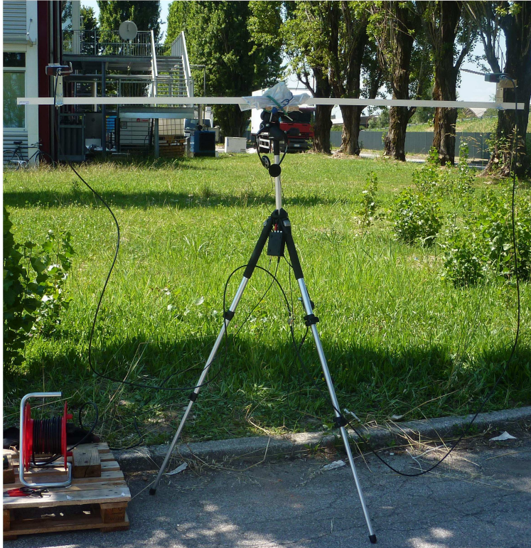
Figure 3.3: The phase interferometer constructed from two identical Yagi-Uda antennae positioned along a baseline perpendicular to the direction of the transmitter (the helicoidal parabolic antenna is in the background, on the top left corner of the picture). The two antennae are connected together with a 180^\circ -phase-shifted cable through a beam adder module, in order to obtain a phase-difference interferometer. They can be mechanically tilted in the horizontal and vertical directions. The center of the interferometer's baseline was positioned where the minimum of the field was measured.
