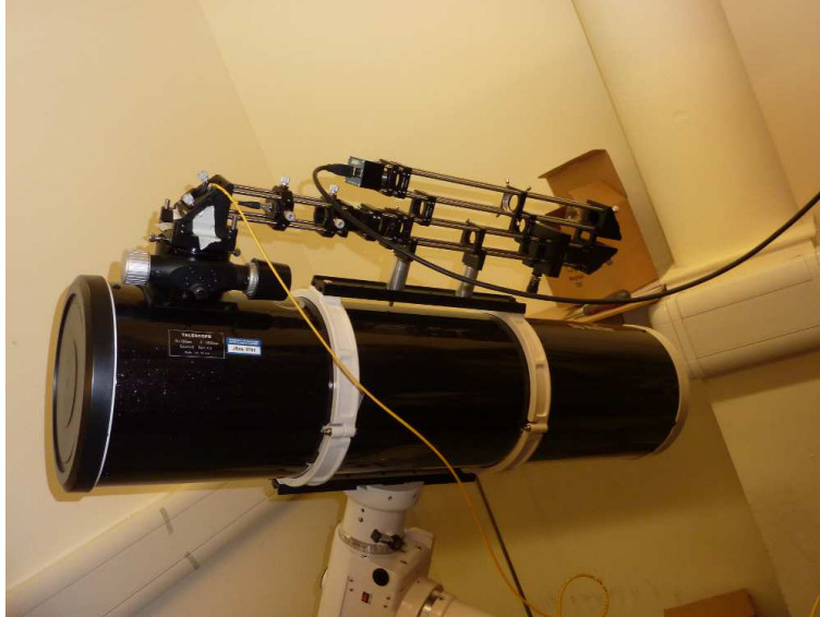
Figure 4.3: The 19 cm telescope we used for the first tests to adapt the OAM mode sorter to an optical telescope. To align the OAM mode sorter, we used a Laguerre-Gaussian beam entering in the sorter through a fiber (the yellow cable).
