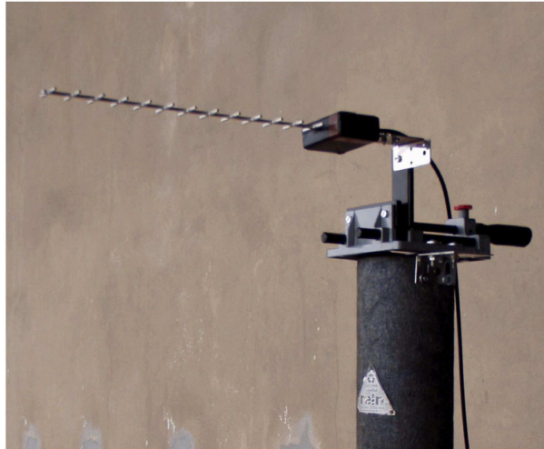
Figure 3.11: One of the two receiving Yagi-Uda antennae of the interferometer mounted on the top of an isolated plastic pillar.
