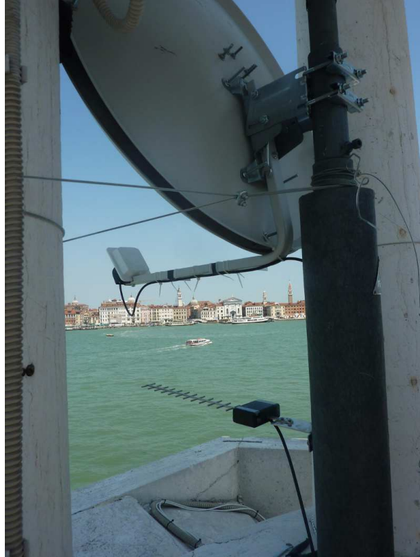
Figure 3.5: The two transmitters located in the lighthouse of San Giorgio island (in front of Palazzo Ducale, at a distance of 442 m). The helicoidal parabolic antenna generates the \ell = 1 signal, while the Yagi-Uda antenna below transmits the \ell = 0 signal.
