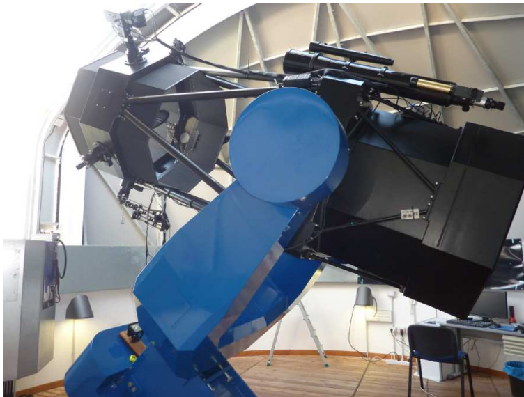
Figure 4.6: The 80cm Newtonian telescope at Celado observatory.
