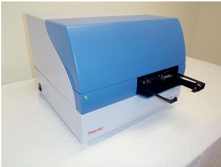
Figure 1. Calibrated automated thrombogram system (CAT) by Thermo Electron. The instrument consists of a 96-well microplate fluorometer and Thrombinoscope™ package.
