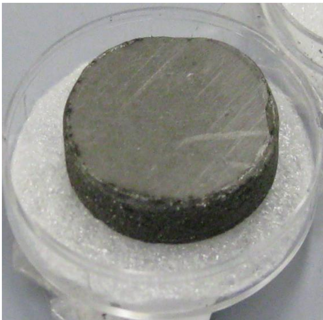
Figure 3.7: Highly Oriented Pyrolytic Graphite (HOPG) Target (Optigraph GmbH Berlin, Germany).
