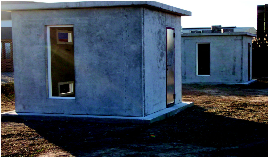
Figure 16: Test cubicles with inclusion of PCM in concrete (a) and results (b) (Castellón et al. , 2007)
