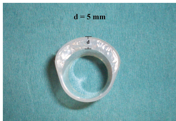
Fig. 15. Axial slice of the EA 4015 Silicone Standoff kit of 5 mm thickness
