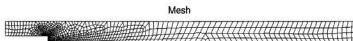
Figure 6.13 Flow over a backward-facing step – Unstructured finite element mesh of the computational domain
