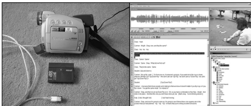
FIGURE 2 Digital video recording equipment: video camera with firewire computer lead, mini DV cassette and Transana transcribing software
