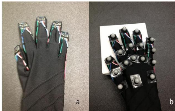
Figure 17. Glove-Based Prototype Device (A) Glove Without Markers (B) Glove With Markers Attached
