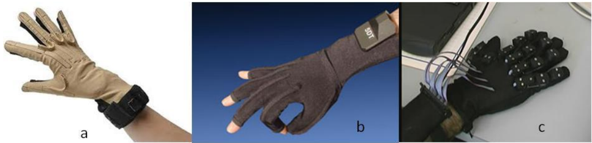
Figure 3. Commercially Available Glove-Based Devices: (a) Cyberglove (b) DataGlove (c) Humanglove
