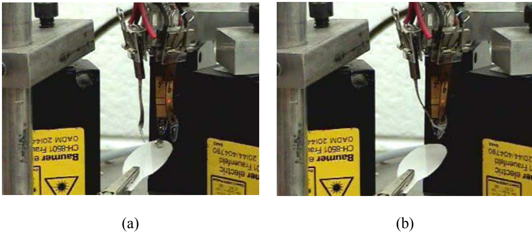
Fig. 1.7 Two steps of gripping motion by IPMC three-finger gripper [35]. Three IPMC strips work as fingers with individual laser sensor for precise position control.
