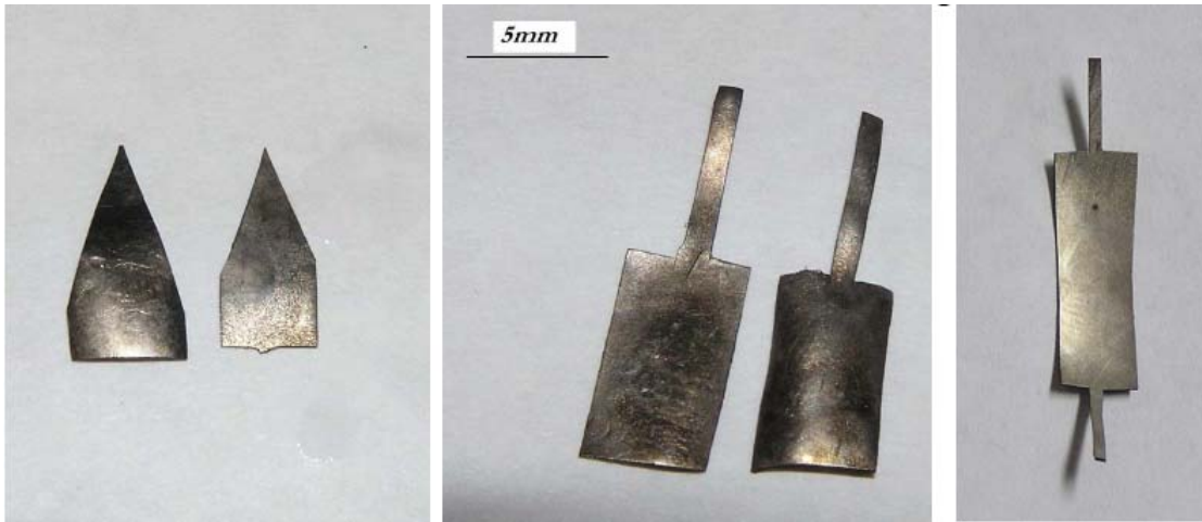
Fig. 2.10 Various shapes of IPMC grippers [60]
