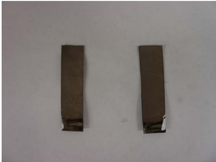
Fig. 2.5 Self-fabricated IPMC strips with burned surface due to external voltage
