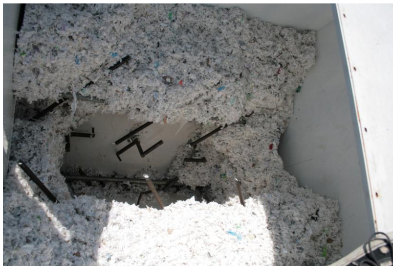
Figure 22. Ratholing and arching of shredded MSW
