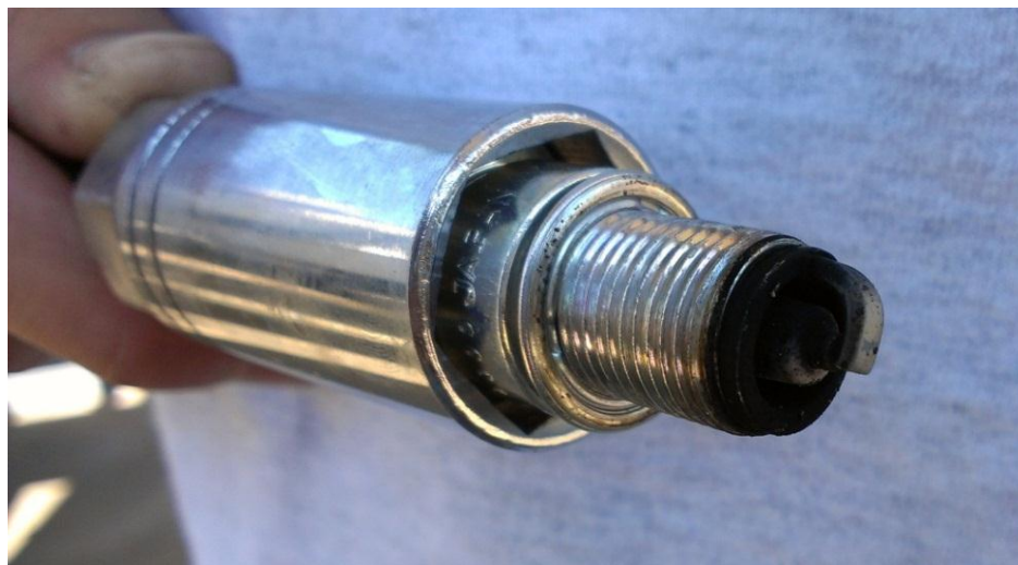
Figure 35. Spark plug condition after synthesis gas–fueled engine operation.
