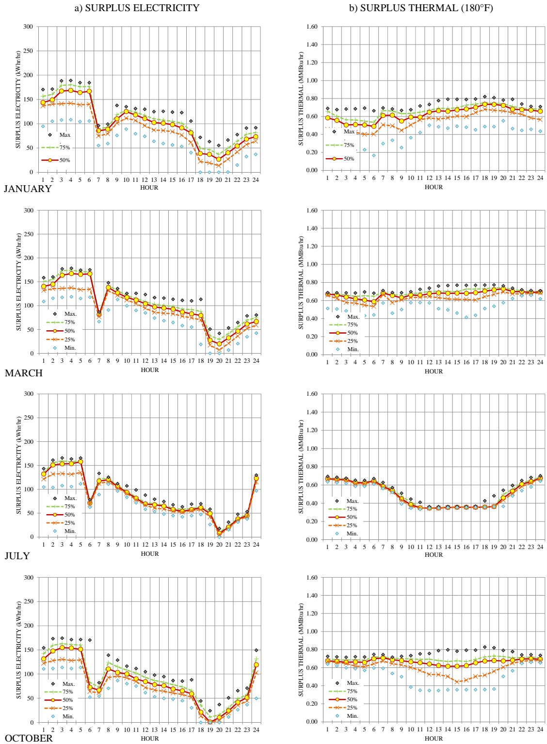
Figure E - 10: Typical Hourly Profiles for Surplus Electricity and Thermal Energy from Option 2
