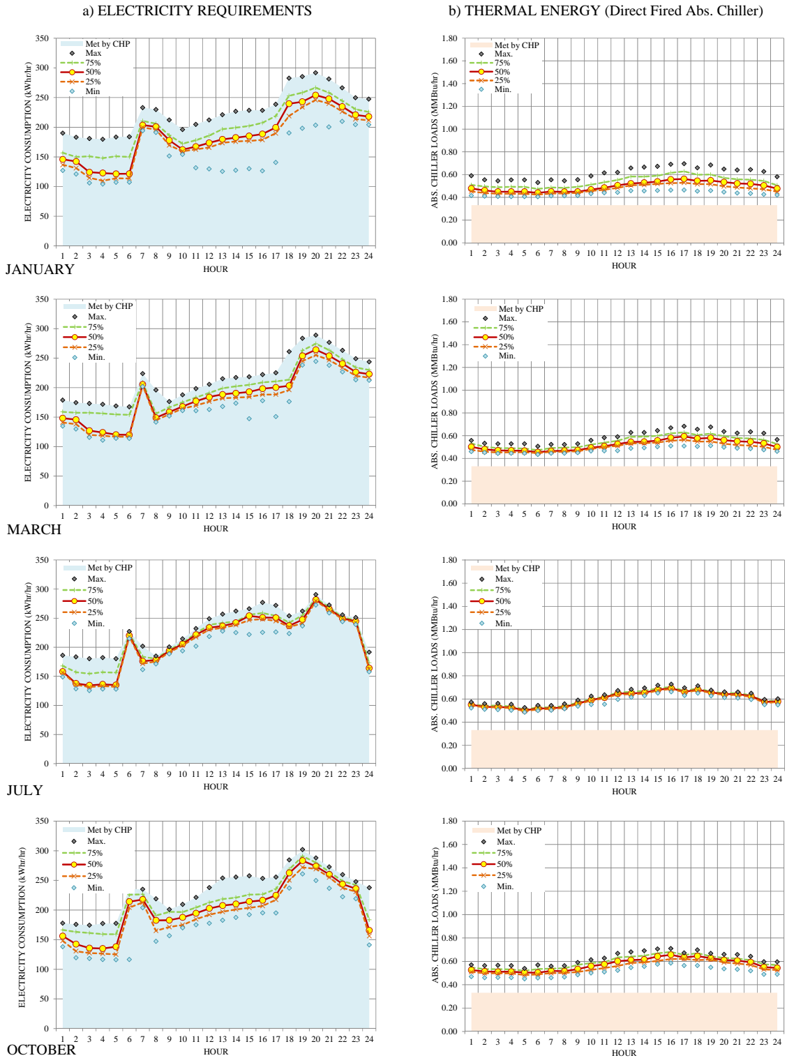
Figure E - 18: Typical Hourly Profiles for Electricity and Absorption Chiller Loads for Option 4
