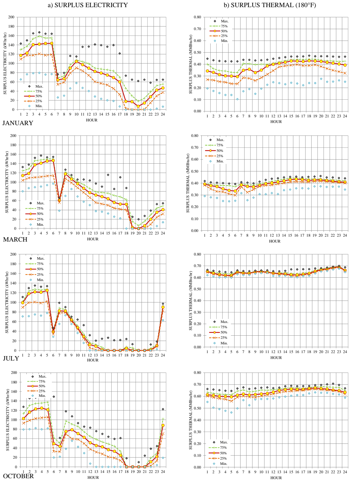
Figure E - 5: Typical Hourly Profiles for Surplus Electricity and Thermal Energy from Option 1
