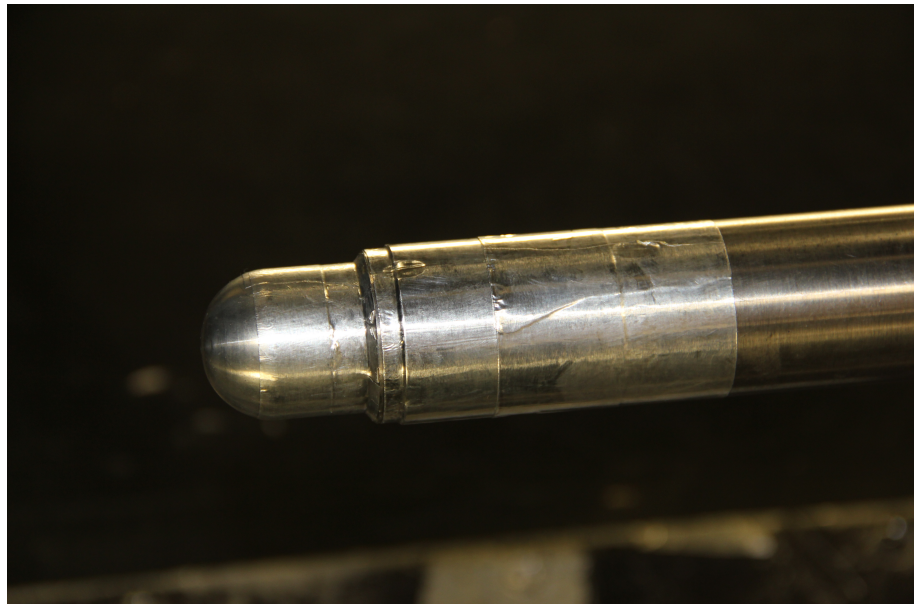
Fig. 14: Ball cover used to keep flow from entering the sting.
