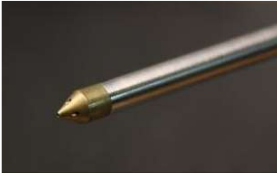
Figure 27 - Five hole probe
