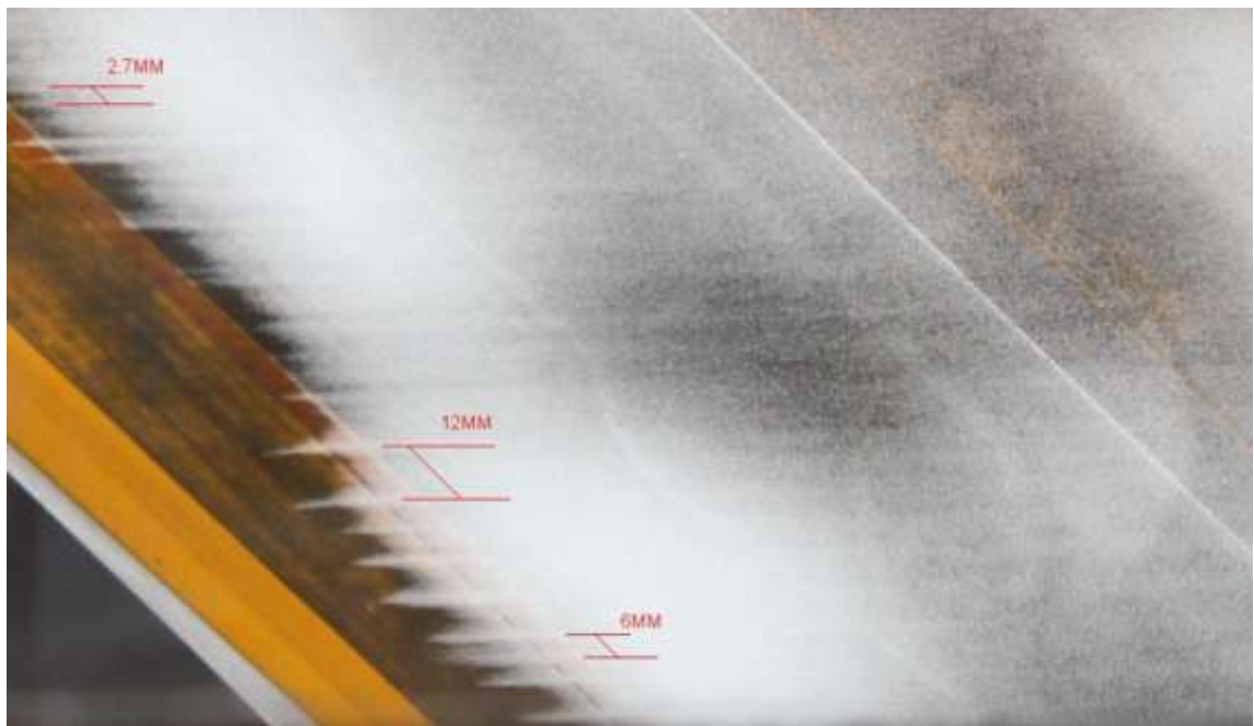
Figure 58 - Wedge and streak pattern at 2.8 \times 10^6 Re_c
