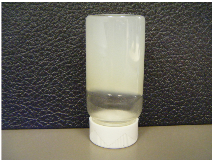
Fig. 5—A Hydrolyzed Polyacrylamide- Polyethylenimine- Dextran Sulfate gel with 7000ppm HPAM, 7000ppm PEI and 3500ppm Dextran Sulfate.
