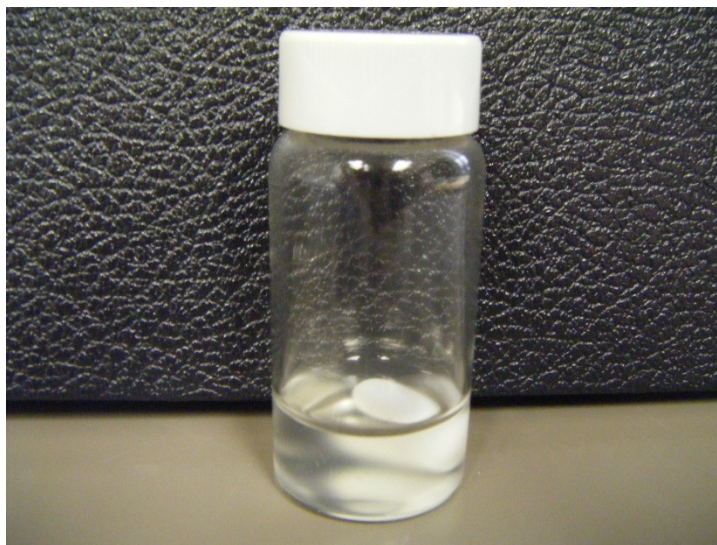
Fig. 4— Polyelectrolyte nanoparticle suspension of Polyethylenimine and Dextran Sulfate.
