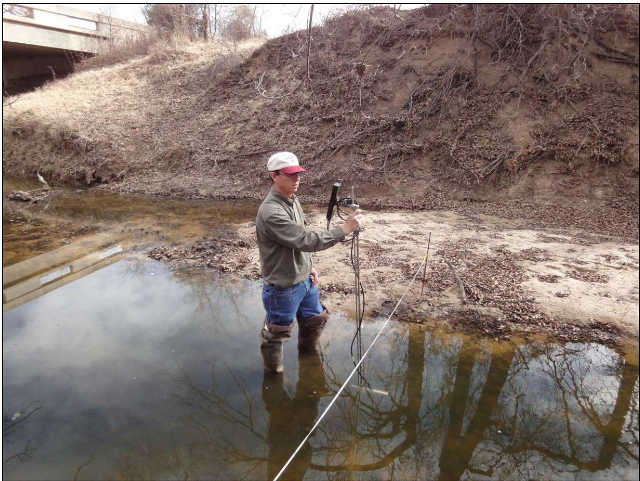
Measuring stream flow with Hach Acoustic Doppler Current (ADC) meter.
