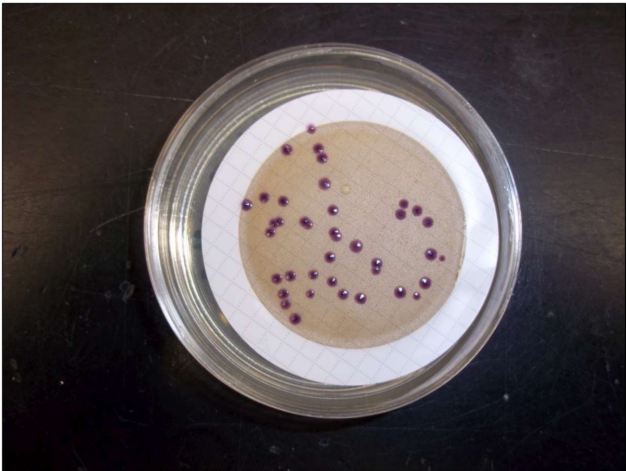
Petri dish with mTEC media and filter positive for E. coli (red colonies).
