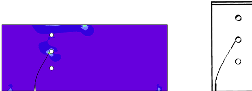
FIGURE 9 (a) Simulated crack trajectory for the single edge cracked plate with three holes stress field distribution for case I (b) experimental trajectory (Ingraffea and Grigoriu 1990)
