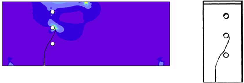
FIGURE 9 (a) Simulated crack trajectory for the single edge cracked plate with three holes stress field distribution for case I (b) experimental trajectory (Ingraffea and Grigoriu 1990)
