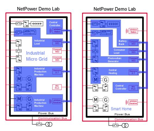
four-quadrant operation and coupled with a DC link and electrical machine units are available. The hardware can be configured in a flexible way by DC and AC coupling to emulate consumers, storage and generators or to build up an island grid. Different machine types are available, e.g. induction machines, synchronous machines or asymmetric permanent magnet out-runners to simulate an EV power train or a domestic or industrial consumer.
