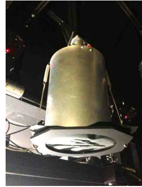
(b) Infrared lamp with color foils mounted on top of the CAVE
