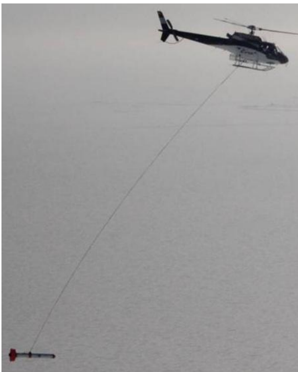
Figure 3: MAiSIE on arctic field campaign close to Barrow Alaska (Photo courtesy David Ball).
