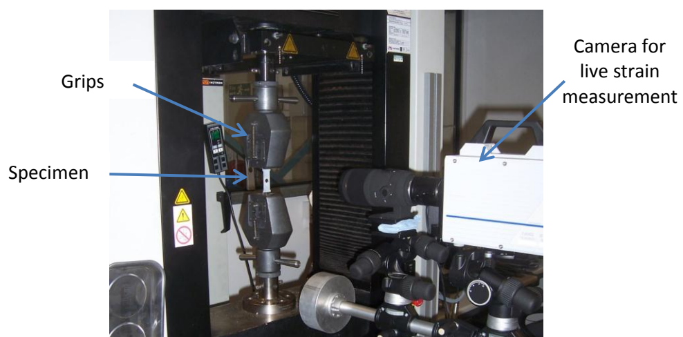
Figure 9 – Low speed Instron 5800R testing machine with DIC setup
