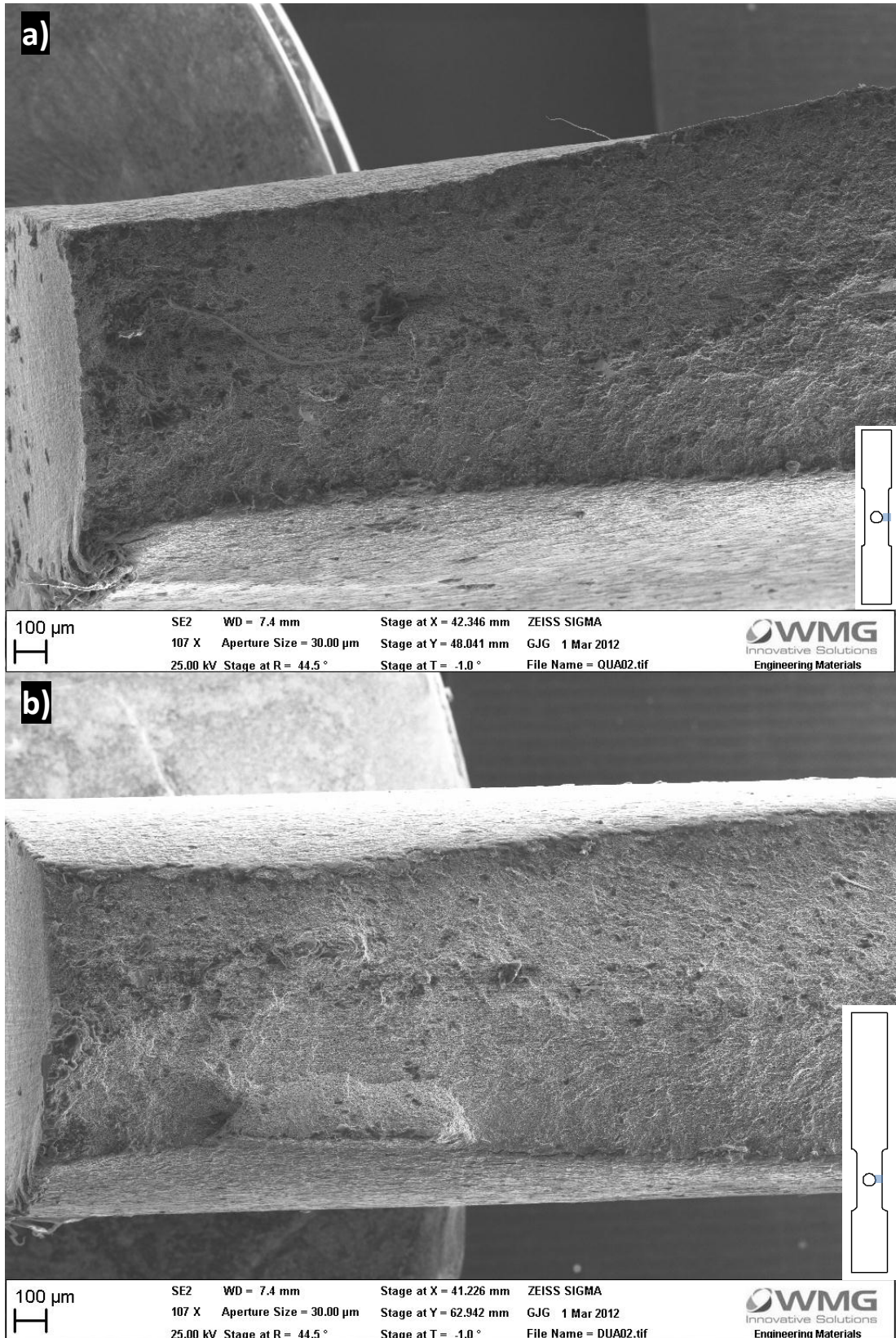
Figure 69 – SEM images of fracture surfaces of DP800 uniaxial fracture specimens, loaded at a) 1 \text{ s}^{-1} and b) 100 \text{ s}^{-1}
